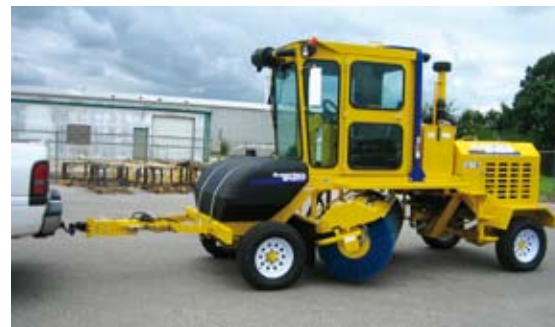
OPTIONAL GUTTER BRUSH Gutter brush has 27 inch brush head with hydraulic power angle, tilt down pressure and float. Brush is mounted to front bumper for better operator visibility and folds up when not in use.
