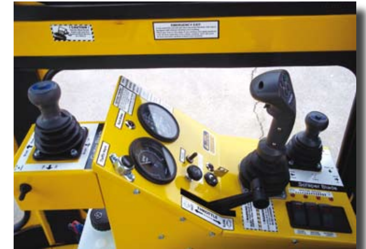
BROOM CONTROLS Electronic joystick control for all broom functions with red LED lights indicating brush speed, full gauge package with tachometer, oil & water gauge, volt meter, fuel gauge and sealed rocker switches with red indicator lights.
